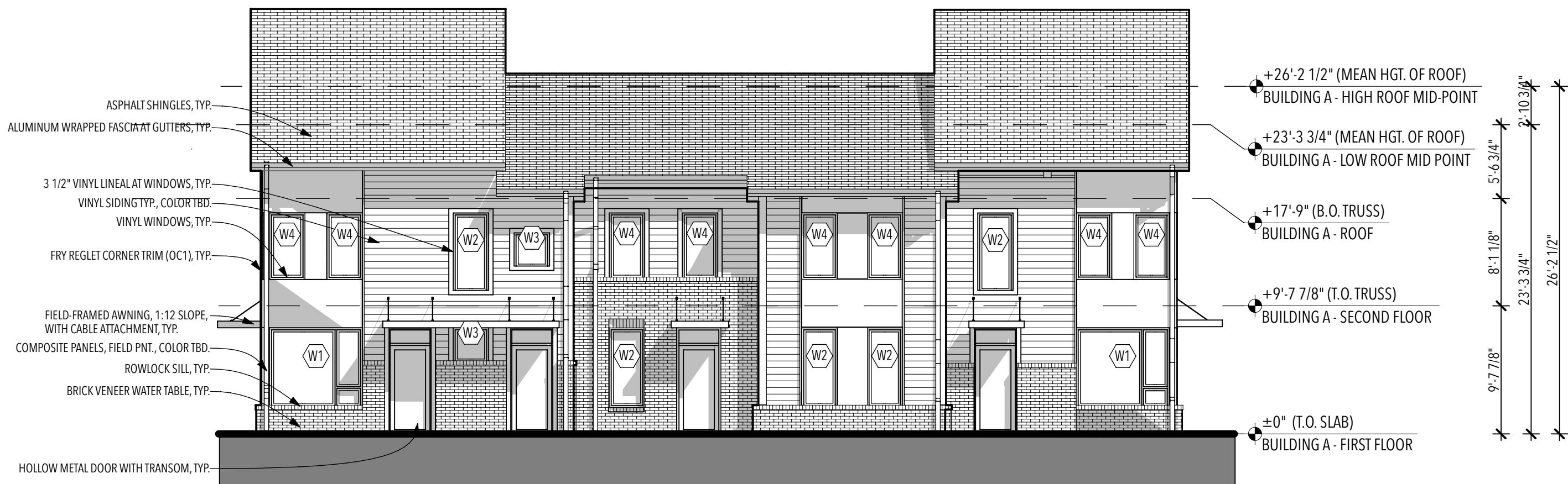
1 BLDG A FRONT ELEVATION ZE-1 SCALE: 1/8" = 1'-0"
