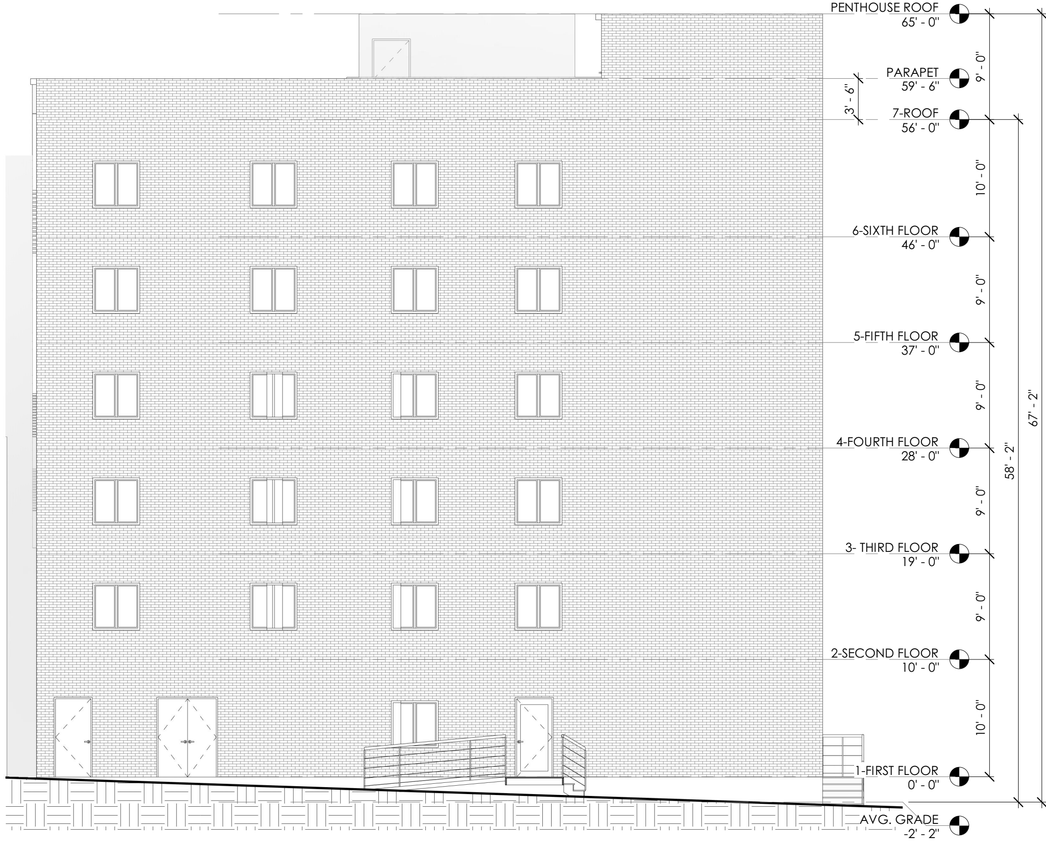
4 Z Front Elevation (Buttonwood st) North SP-1 1/8" = 1'-0"
