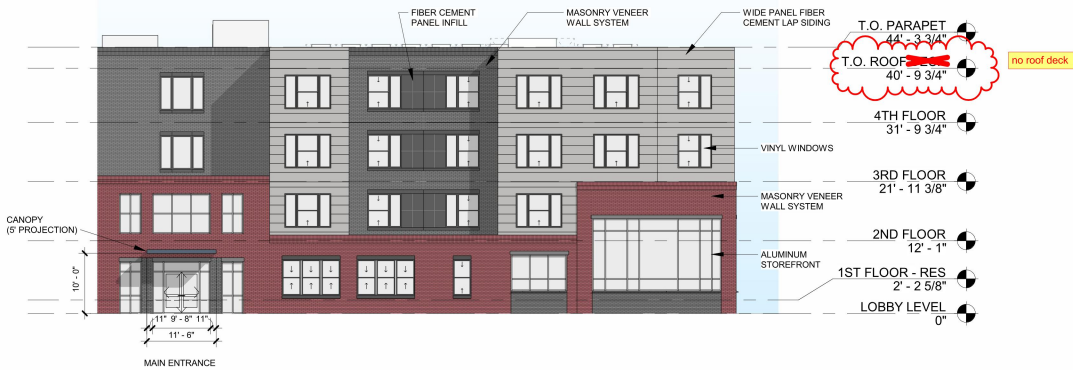
1 LOCUST AVE (NW) ELEVATION 1/16" = 1'-0"
