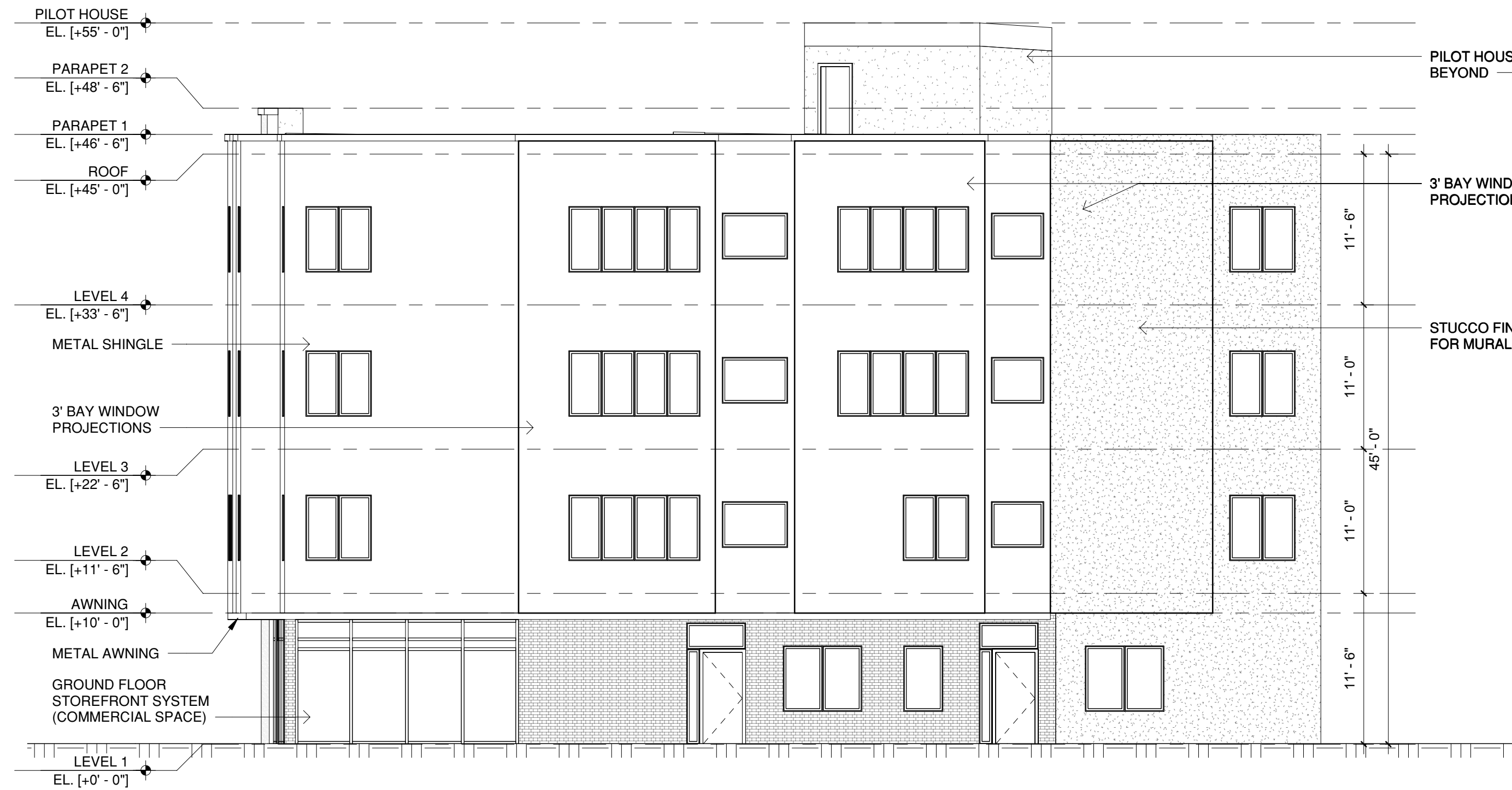
2 WEST ELEVATION (40TH STREET) SCALE: 1/8" = 1'-0"
