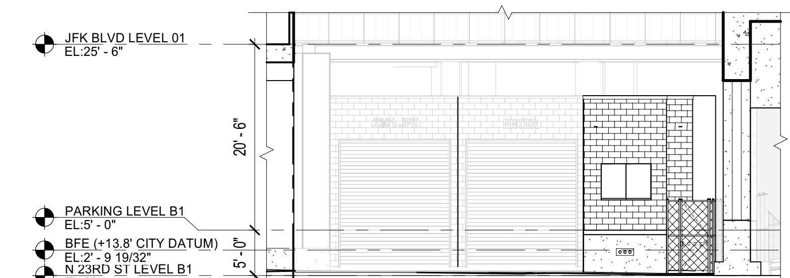
5 23RD STREET PARKING ENTRY ELEVATION - WEST SCALE: 3/32" = 1'-0"
