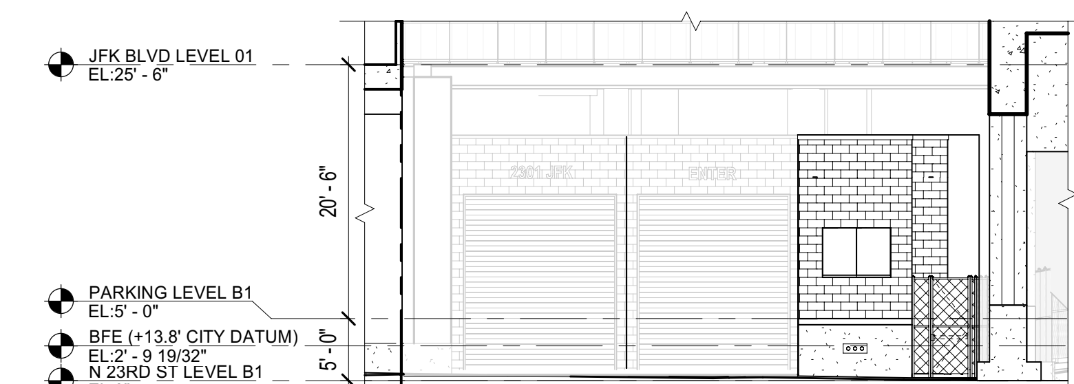
5 23RD STREET PARKING ENTRY ELEVATION - WEST SCALE: 3/32" = 1'-0"
