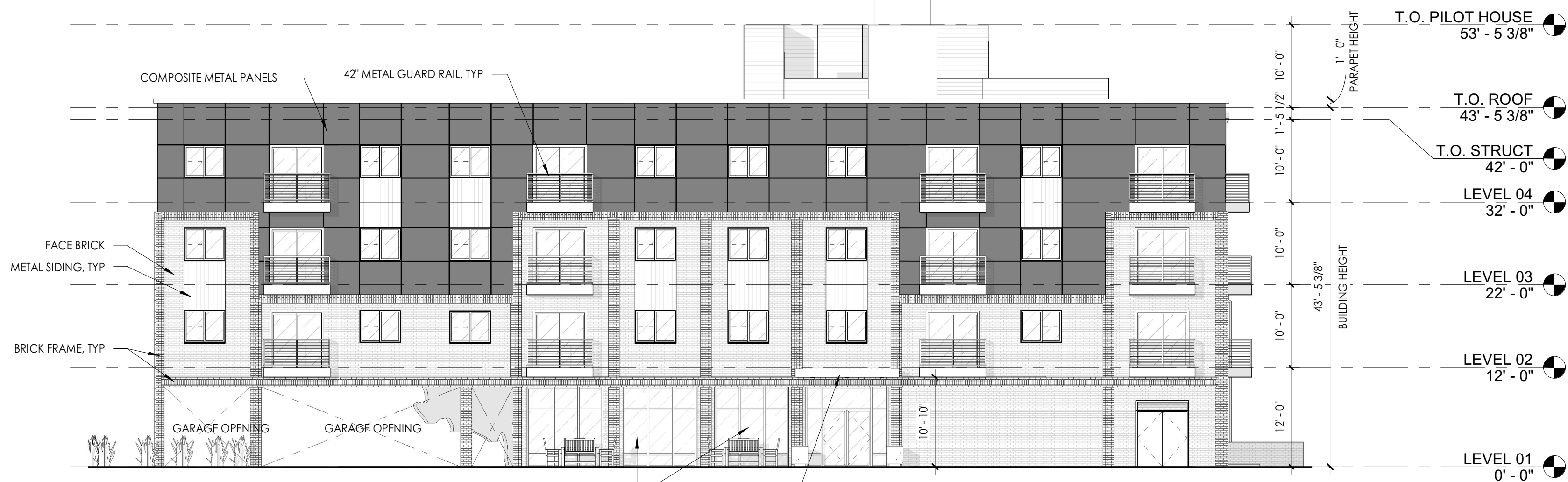
1 | SOUTH ELEVATION (EASTBURN AVE) - ZONING Z003 | 3/32" = 1'-0"
