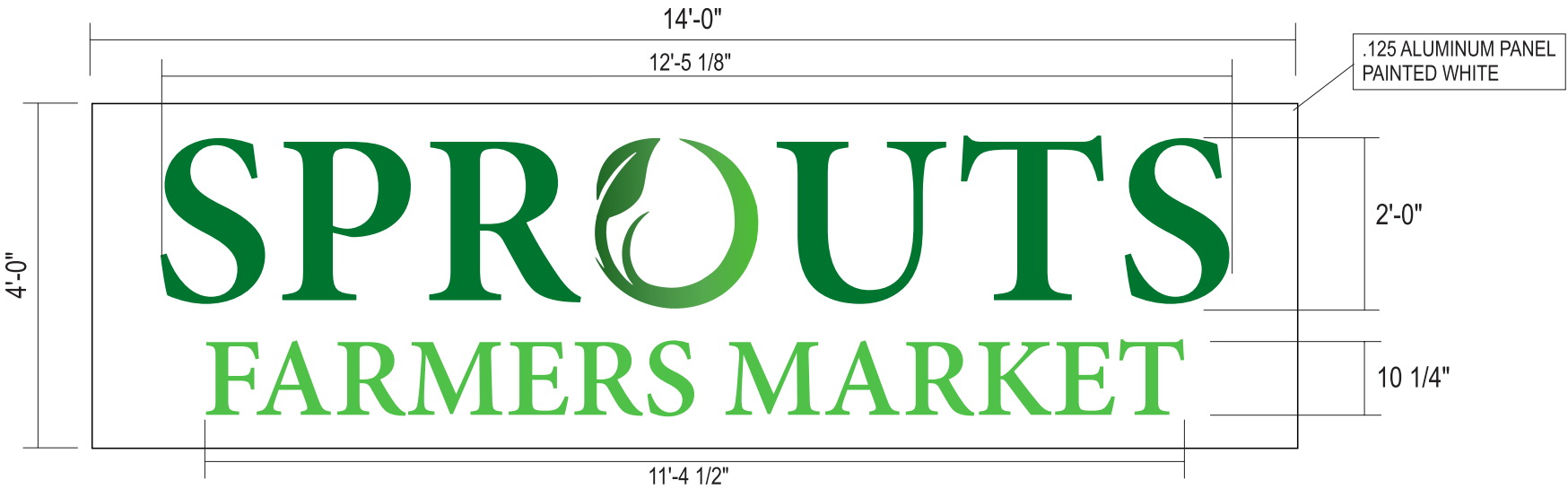
CHANNEL LETTERS ON ALUM. B/G PANEL - "GREEN DAY/GREEN NIGHT" SCALE: 3/8"=1'-0"
