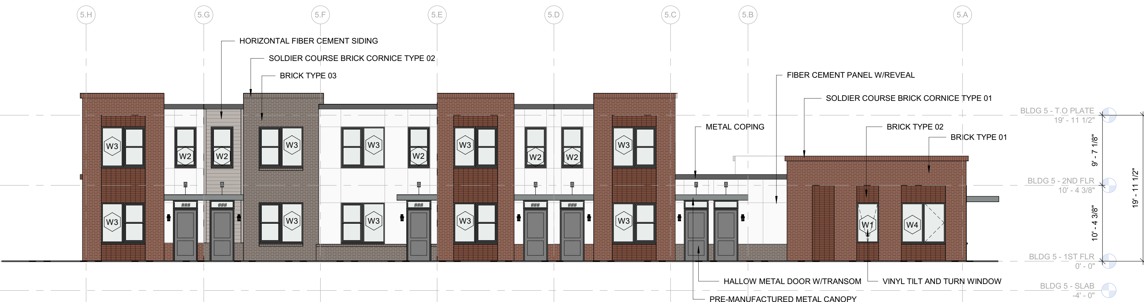
1 BLDG 5 EAST ELEVATION 1/8" = 1'-0"
