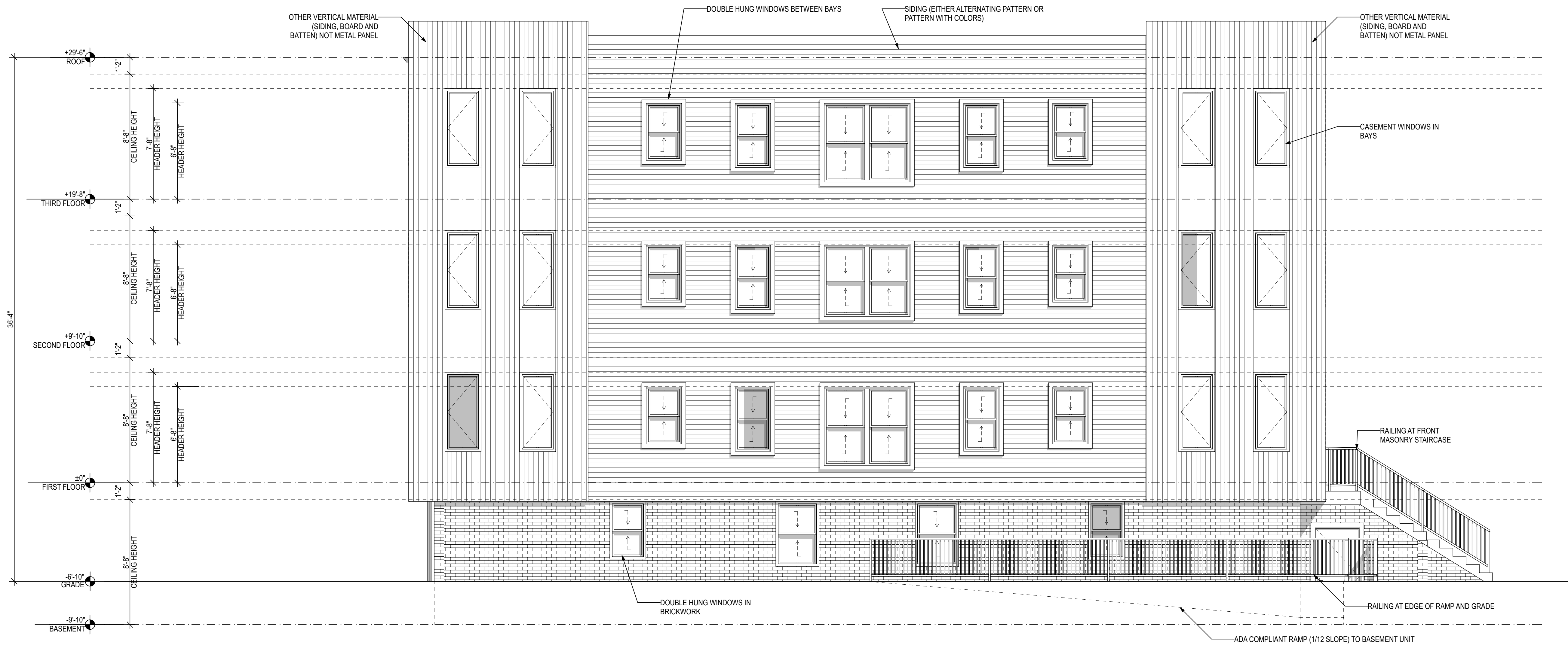
SIDE ELEVATION - NORTH PARK AVE SCALE: 1/4" = 1'-0"
