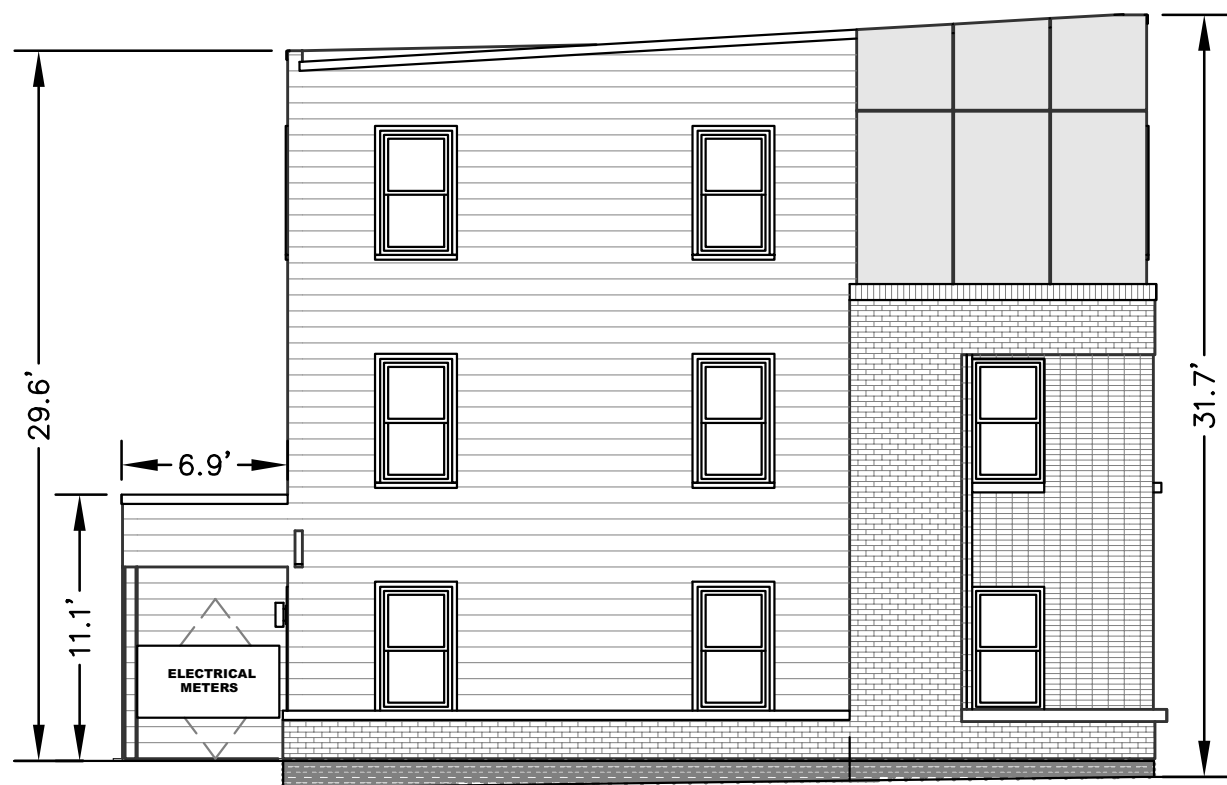
BUILDING 2 NORTH ELEVATION
